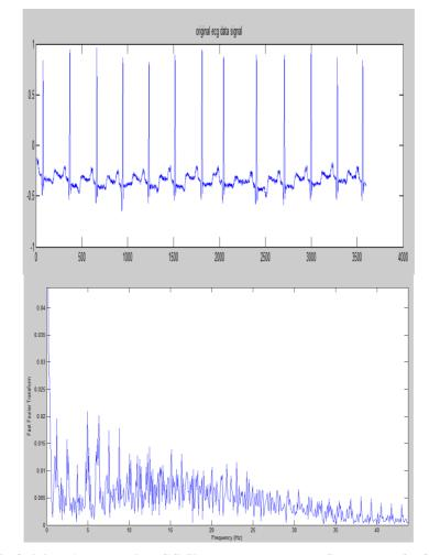
Figure 2: Original Arrhythmia ECG Signal and Frequency Spectrum. of ECG Signal
